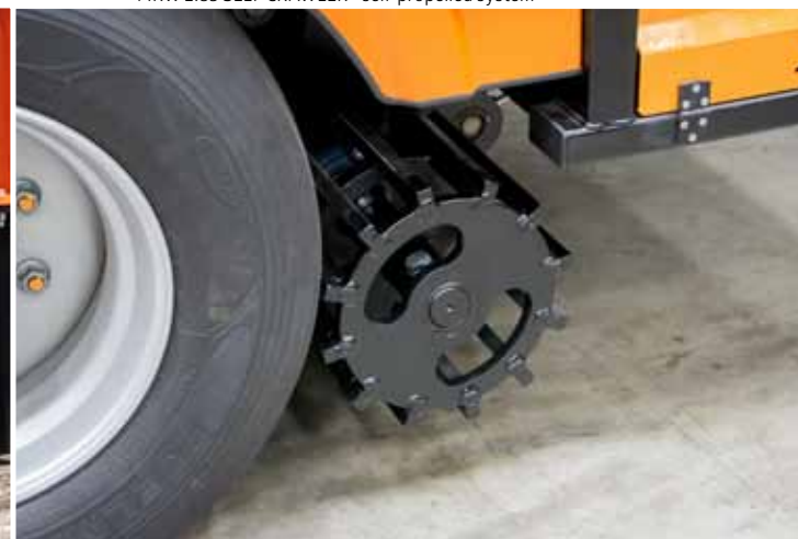
MRW 2.85 SELF CRAWLER - self-propelled system
