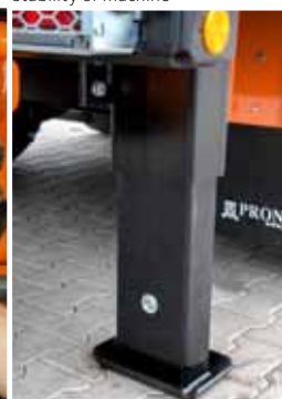
Hydraulic support legs ensures stability of machine
