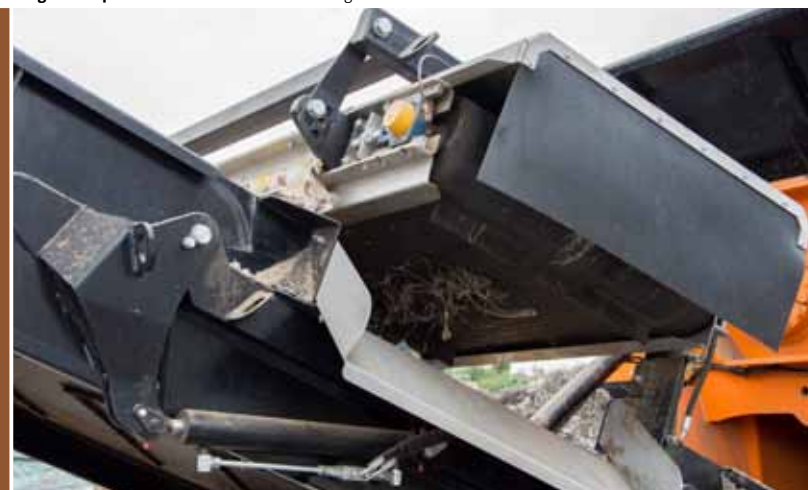
Magnetic separator for extraction of ferromagnetic materials.
