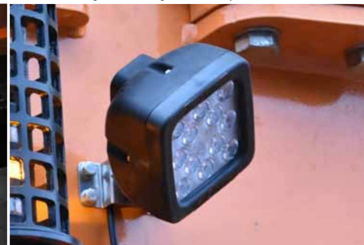
Working area additional lights increase safety near the machine
