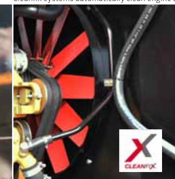
Cleanfix systems automatically clean engine and oil hydraulics radiators
